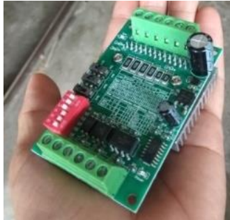
Gambar 4. Motor driver TB6560
