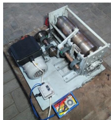
Gambar 2. Model cara kerja mesin laminating
