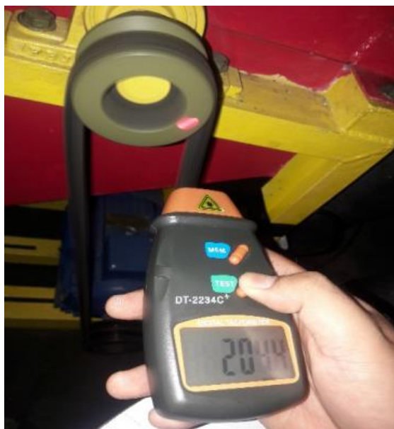
Figure 3. Measuring Rotating Velocity of Pulley of Blade Shaft by Digital Laser Tachometer
