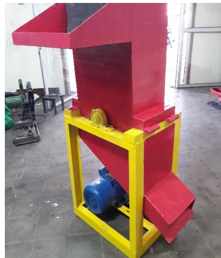
Figure 1. Plastic Bottle Crushing Machine
