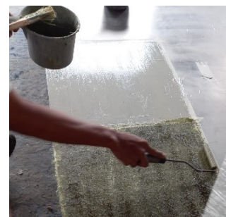
Gambar 1. Proses hand lay up
