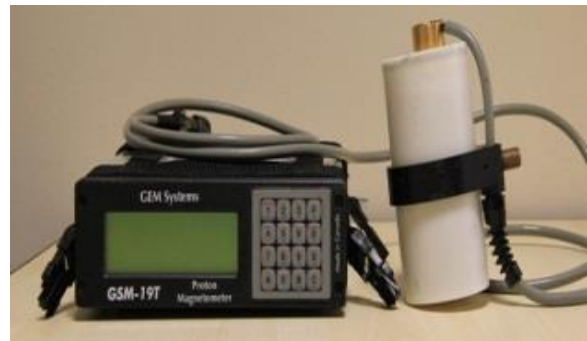
Gambar 2. PPM (Proton Precession Magnetometer) (a) tipe Geometrics G-856, (b) tipe GEM GSM-19T.
