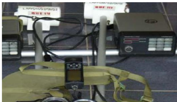
Gambar 2. PPM (Proton Precession Magnetometer) (a) tipe Geometrics G-856, (b) tipe GEM GSM-19T.
